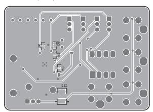
Figure 5: Example PCB Layout.
