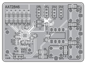
Figure 6: AAT2846 Evaluation Board Layout Top Side.
