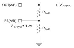
To select appropriate resistor values, first choose  $R_1$  such that the feedback network bias current is less than  $10\mu A$ . Then, according to the desired  $V_{OUT}$ , calculate  $R_1$  according to the equation below. An example calculation follows.
