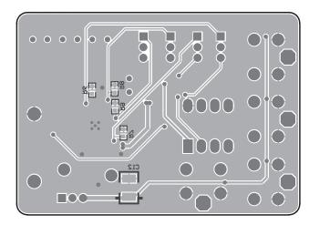
Figure 7: AAT2846 Evaluation Board Layout Bottom Side.
