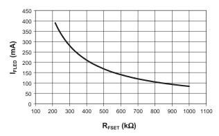
Figure 4: Maximum Flash LED Current vs. R<sub>FSET</sub>.
