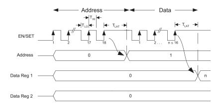
Figure 1: AS<sup>2</sup>Cwire Serial Interface Timing.
