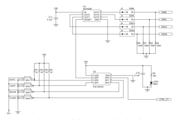
Figure 9: MCU and I/O Expander Section Schematic.
